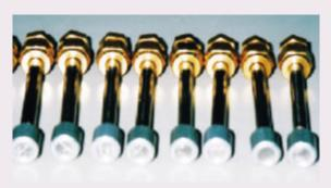
Figure 1 Tube-type diffusive sampler
