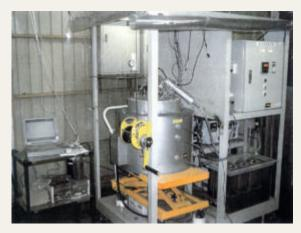
Figure 2.2-2 Batch type pyrolysis reactor
